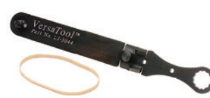
3044 VERSATOOL™ Locates holes as well as starts and tightens hex nuts onto rail bolts. Drives 5/16" rail bolts and tightens 1/2" hex nuts. Also used to locate 1/4" pilot hole on handrails & rail drops for attaching to Connect-A-Kit® handrail fittings.
