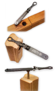
3044 VERSATOOL™ Locates holes as well as starts and tightens hex nuts onto rail bolts. Drives 5/16" rail bolts and tightens 1/2" hex nuts. Also used to locate 1/4" pilot hole on handrails & rail drops for attaching to Connect-A-Kit® handrail fittings.
